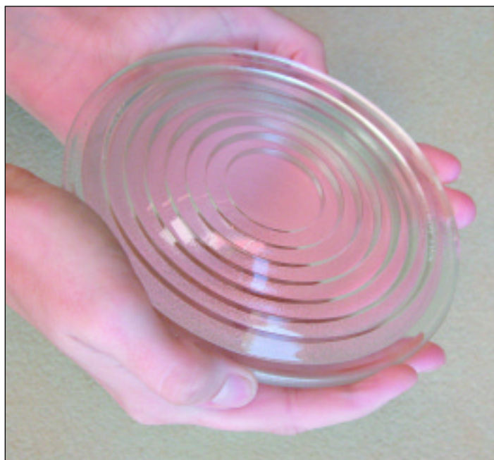
The concentric design of a Fresnel lens gives the instrument its characteristic softly focused, diffuse light.
